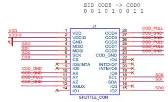
BME680 shuttle board electrical layout
