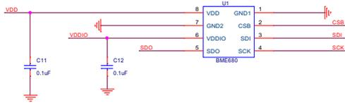
Unless mentioned in value, all resistor and capacitor could use 0603
